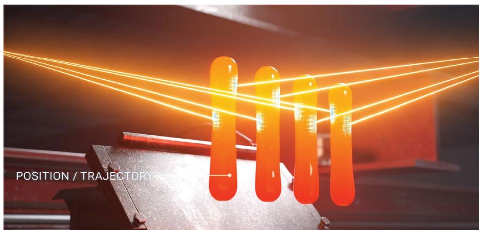
The high speed matrix cameras can still monitor partially obscured gobs.
